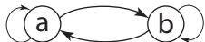
FIG. 6: Representation of the coarse-grained two-state system as a discrete finite-state model with forced transitions on every interval of length \Delta t .
